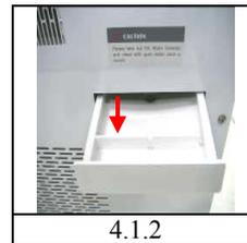
After machine running for a period of time ,clean up the dust that may store up in the water collector .when cleaning,take out out water collector from the back (diagram 4.1.2) .Clean and replace back to original position. Attention: insert the water collector along its track until its original position.
